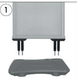
**GB** Place the springs into the holes of the plastic base.
